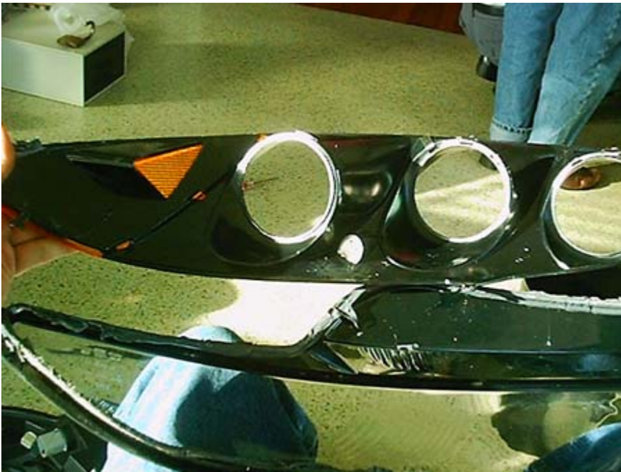
The inside is held in by several screws. Take them all out and then you can pull the black middle piece out..
